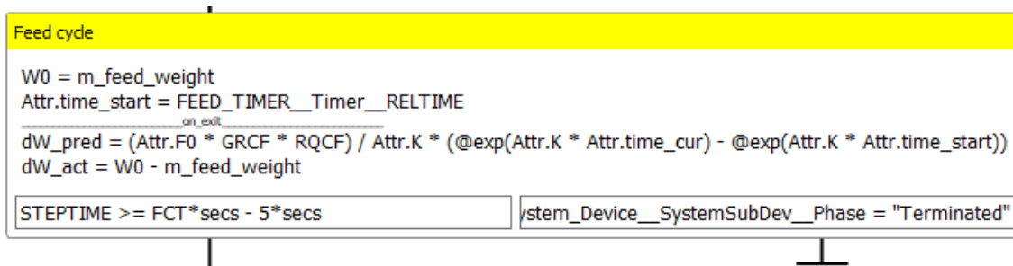
Figure 14: Calculation of the predicted weight decrease (parameter dW_pred ), based on the gravimetric feed correction factor and the exponential feed equation integrated throughout a full feed cycle, and calculation of the actual weight decrease (parameter dW_act ), based on balance measurements at the start and end of a feed cycle.
